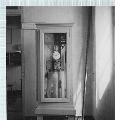
Figure 3. View of the recording drum and clock of the mechanical floating tide gauge at Dakar (SHOM, 1959).
