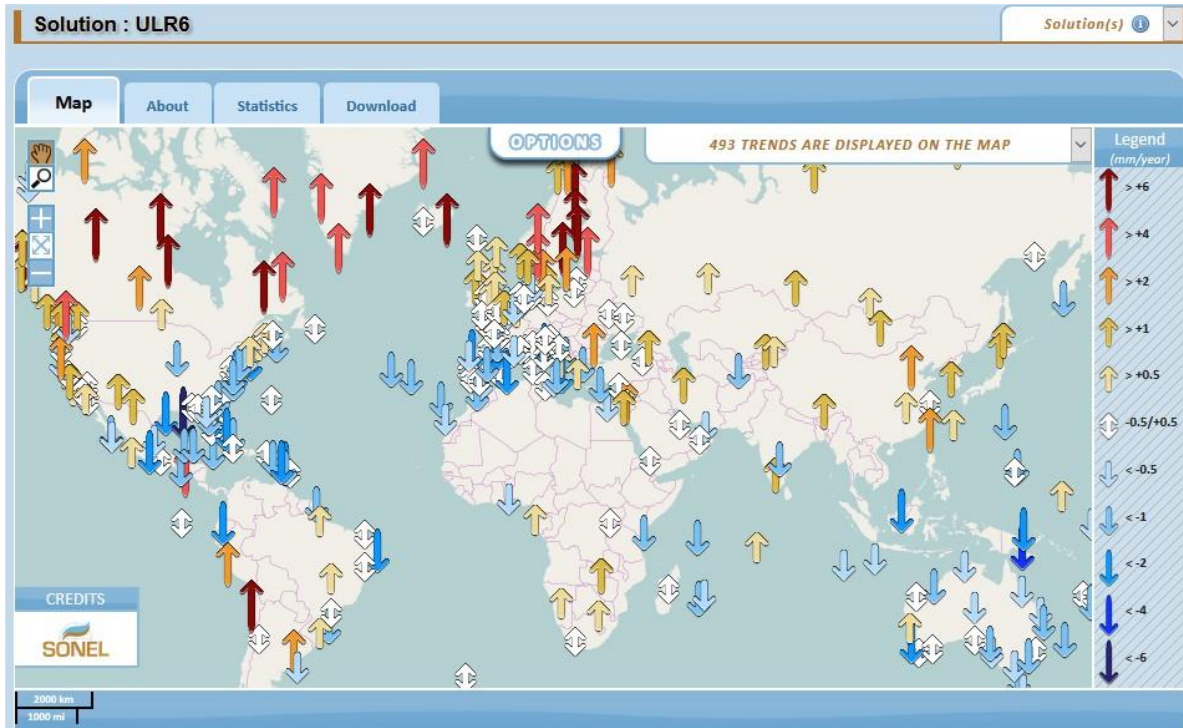
Figure 7: Display on a web-based clickable map of the GNSS vertical velocities from ULR6 solution http://www.sonel.org/-Vertical-land-movement-estimate-.html?lang=en
