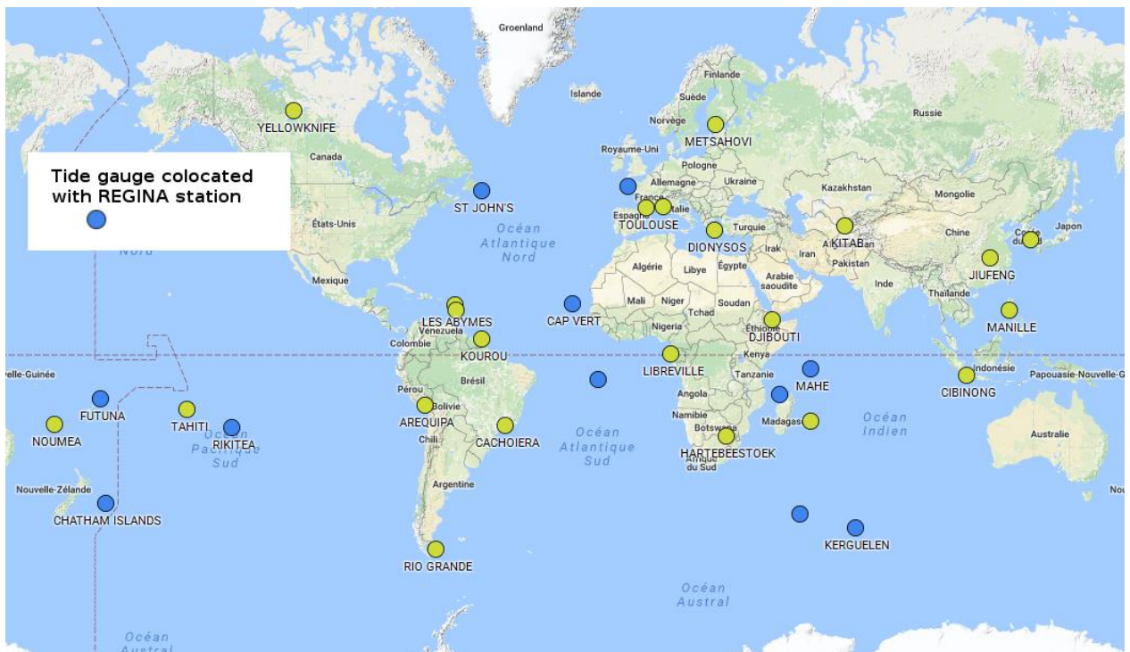
Fig. 5 Map of REGINA stations co-location with Tide Gauges (source : T.Donal, IGN, December 2016)
